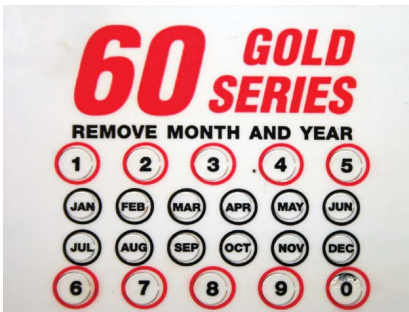
FIGURE 5-3 The battery sticker will usually have the date the battery was sold, plus additional information.
