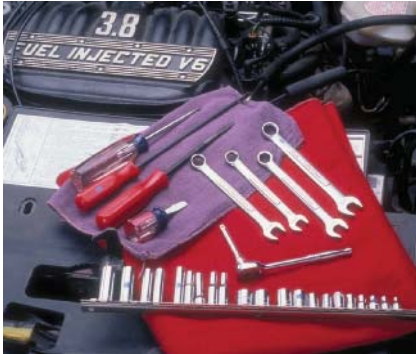
P28-1 Tools required to replace the servo assembly: fender covers, screwdriver set, combination wrench set, ratchet and socket set.
