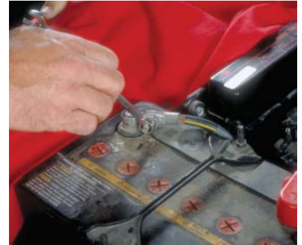
P6-3 Disconnect the fuse that powers the circuit being repaired. Note: If the circuit is not protected by a fuse, then disconnect the battery.
