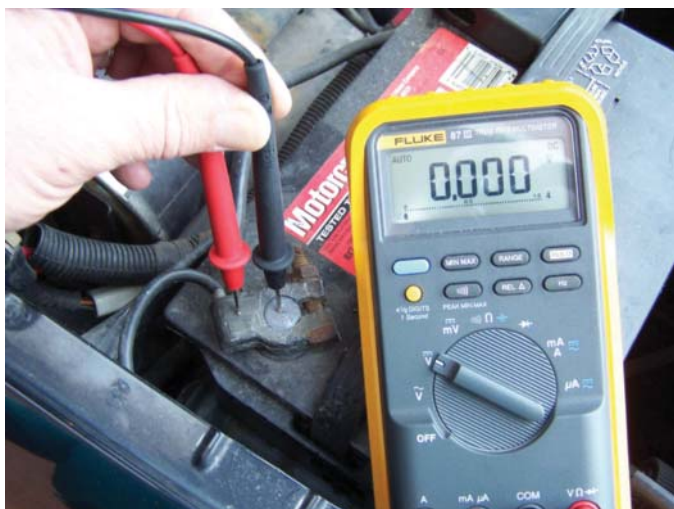
FIGURE 5-7 Voltmeter connections for the battery terminal test.
