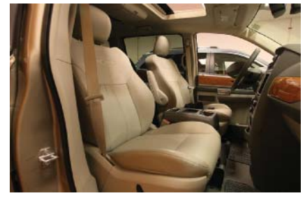
P30-3 Make sure the seat is empty and is in its full rearward position, with the back rest in a normal upright position.
