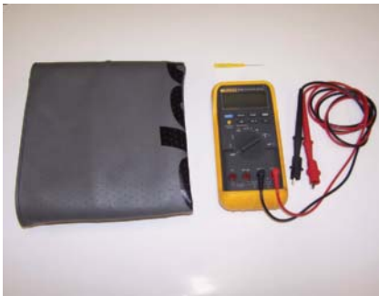
P3-1 The tools required to perform this task include voltmeter, backprobing tool, and fender covers.
