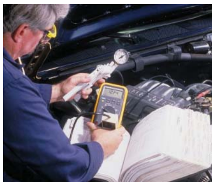
P19-8 Apply 15 in. Hg to the MAP sensor and compare the reading to specifications.
