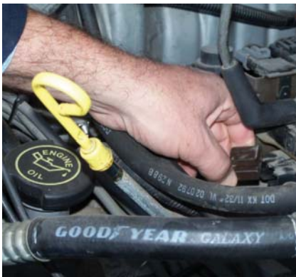
P4-4 To conduct a voltage drop test, current must flow through the circuit. In this test, the ignition system is disabled and the engine is cranked using a remote starter switch.
