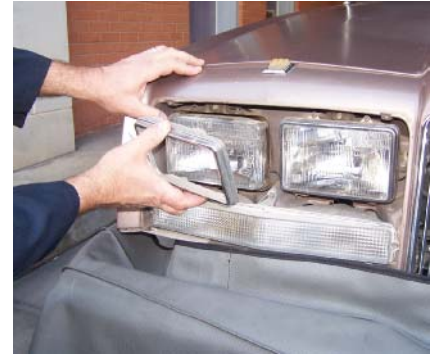
P15-3 Remove the retaining ring screws and the retaining trim. Do not turn the two headlight aiming adjustment screws.
