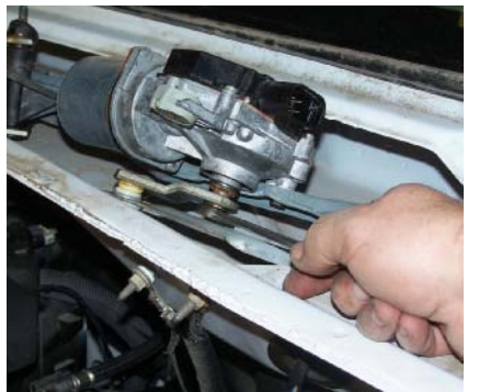
P24-6 Remove the linkage from the motor.
