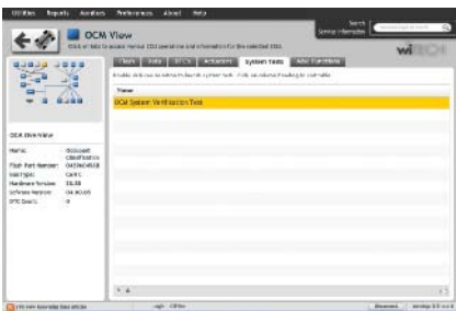
P30-4 Use the scan tool to access the "OCM Verification" screen and follow the instructions to begin the test.
