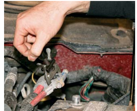
P9-6 Loosen the clamp bolt for the positive cable and use the terminal puller to remove the cable. If the battery has a heat shield, remove it.
