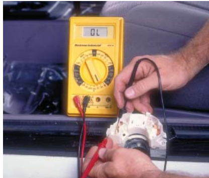
P16-14 The circuits between terminals 196 and 13, and 196 and 12, should be open in the low-beam position.
