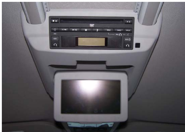
FIGURE 14-103 Flip-down, roof-mounted, DVD monitor.
