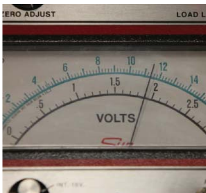
P8-8 Read and record the voltmeter while applying the load for 15 seconds.
