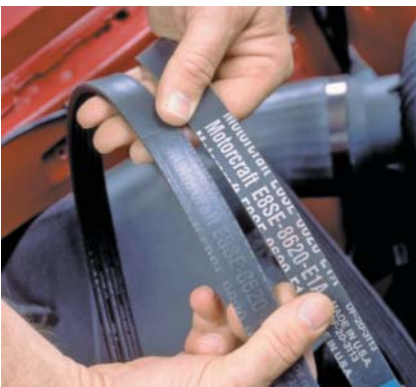
P13-7 Confirm that the new belt is the same size as the old one.
