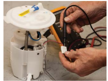
P23-3 Connect the negative test lead DMM to the ground terminal of the sender unit.
