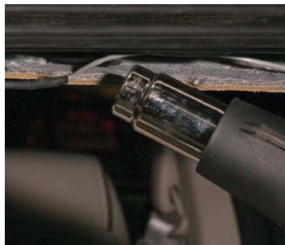
PS7-13 Locate the heat shrink tube over the splice area and use the heat gun to shrink the tube over the cable.
