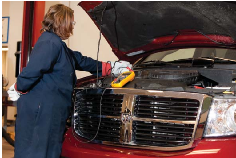
FIGURE 1-28 Follow the “one-hand” rule while testing the high-voltage system of an HEV.
