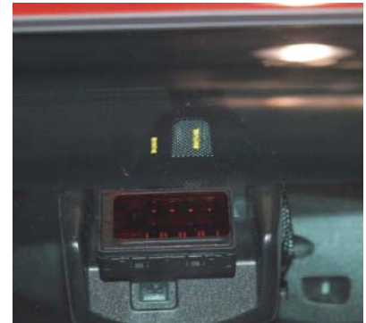
P22-3 Divide the measurement in half and mark that dimension near the lower edge of the tint band using a grease pencil.
