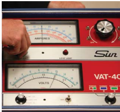
P8-5 Confirm that the meter reads zero amperes. If needed, zero the ammeter.
