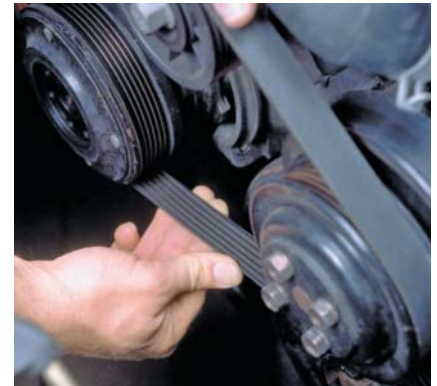
P13-12 Measure the deflection of the belt or use a gauge as recommended by the manufacturer.
