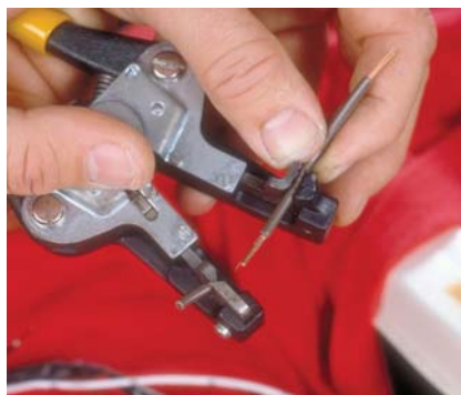
P6-8 Using the correct size stripper, remove 1/2 inch (12mm) of insulation from each end of the replacement wire.
