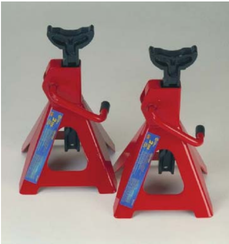
FIGURE 1-8 Jack stands should be used to support the vehicle after it has been lifted by a floor jack.
