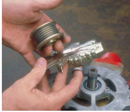
P14-14 Remove the pulley attaching nut, flatwasher, drive pulley, fan, and fan spacer from the rotor shaft.
