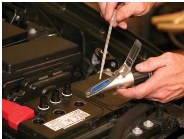
FIGURE 5-15 Placing a sample of electrolyte onto the refractometer's slide.
