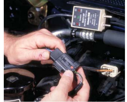
P19-3 Connect the MAP sensor connector to the harness connector.
