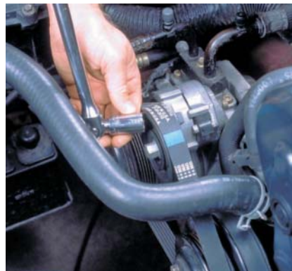
P13-14 Tighten the fasteners to the proper torque specifications.
