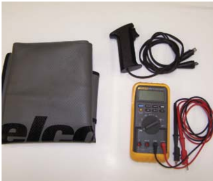
P4-1 Tools required to test for excessive resistance in a starting circuit are fender covers, a DVOM, and a remote starter switch.
