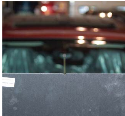
P22-14 While sighting through the V-notch in the upper edge of the calibration target, move the target left or right to align the target to the camera centerline marks on both the windshield and the rear glass.
