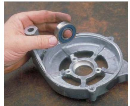
P14-18 Remove the front bearing from the housing. NOTE: It may be necessary to use an arbor press to remove the bearing if it does not slide out.
