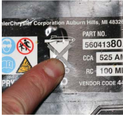
P8-2 Determine the rating on the battery's label and figure the load test specification.
