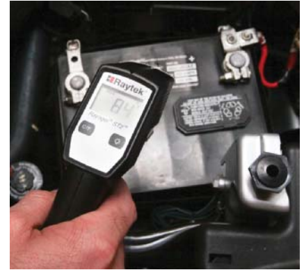
P8-3 Determine the temperature of the electrolyte. If the case is sealed, measure the temperature of the case.
