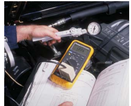
P19-6 Connect a hand vacuum pump to the MAP sensor and supply 5 in. Hg. Observe the MAP sensor reading and compare to specifications.
