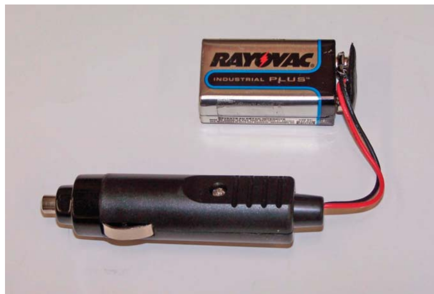
FIGURE 2-38 A memory keeper will keep the computer memories operational while the battery is disconnected.
