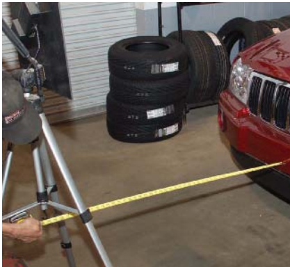
P22-13 Locate the calibration target 50 inches (127 cm) in front of the vehicle measuring from the foremost center of the front fascia.
