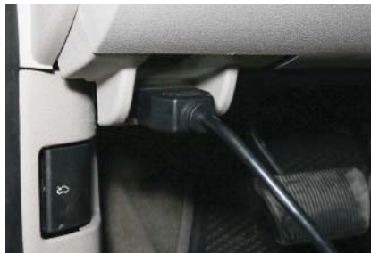
P30-2 Connect the scan tool and check for active battery voltage, OCM internal failure, or communication DTCs. Correct any of these conditions before continuing.
