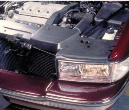
P27-10 Listen for the relay to click. Then the light and horn circuits should be activated.
