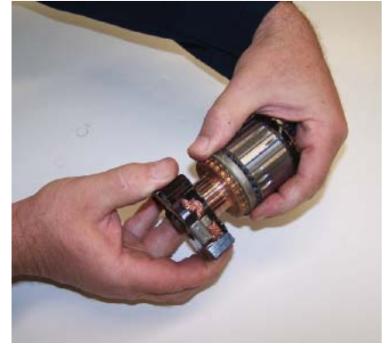
P11-12 Separate the brush assembly from the armature.
