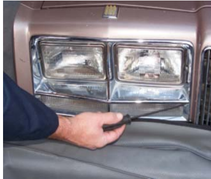
P15-2 Sealed-beam headlight replacement usually requires the removal of the bezel. Some vehicles may require that the turn signal light assembly be removed before the headlight is accessible.
