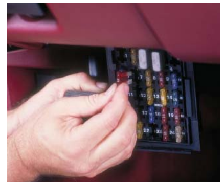
P29-6 Remove the SIR fuse from the fuse box. Wait 10 minutes to allow the reserve energy to dissipate.
