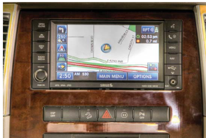
FIGURE 14-105 Navigational system monitor and controls.
