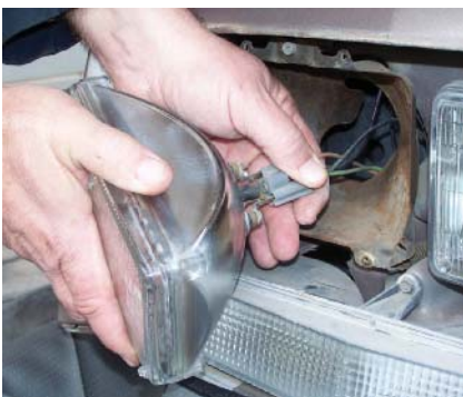
P15-8 Install the wire connector onto the new headlight's connector prongs.
