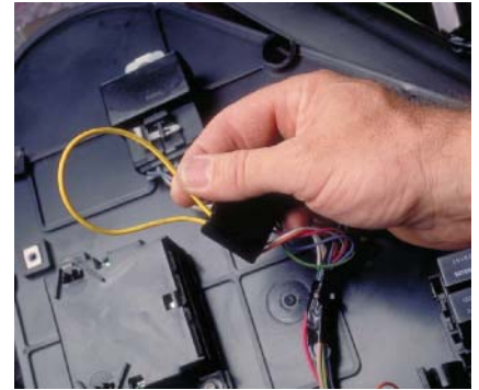
P27-3 Connect the jumper wire between terminals A and B. The horns should sound.
