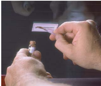
P26-5 Apply the grid repair material to the repair area using a small stick.
