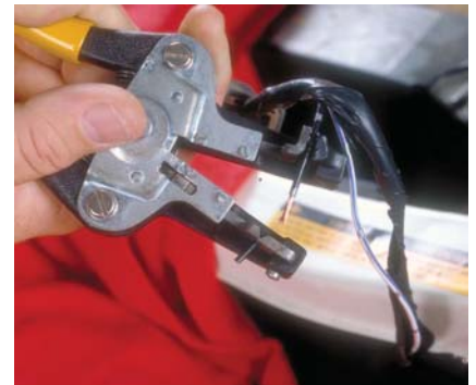
P6-6 Using the correct size stripper, remove about 1/2 inch (12mm) of the insulation from both wires. Be careful not to nick or cut any of the wires.
