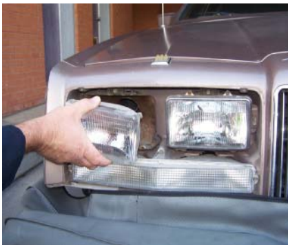
P15-4 Remove the headlight from the shell assembly.
