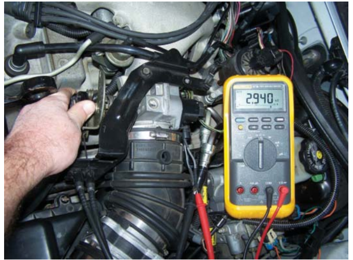
FIGURE 3-30 Testing continuity between terminals A and B of a potentiometer while the wiper is being moved.
