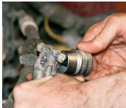
P9-14 Use the terminal cleaning tool to clean the cable.
