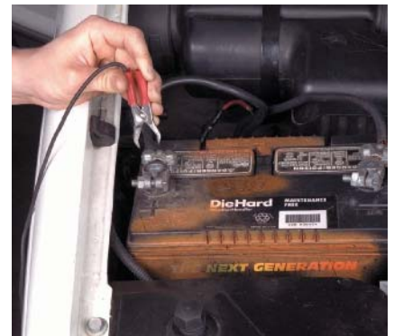
P17-3 If required, connect the scan tester power cables to the vehicle's battery terminals, observing polarity.
