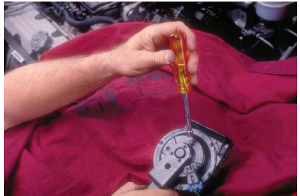
FIGURE 14-3 Horn pitch adjustment screw.
