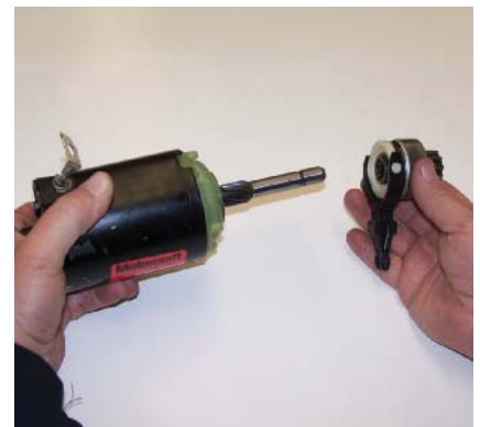
P11-6 Remove the drive from the output shaft.
