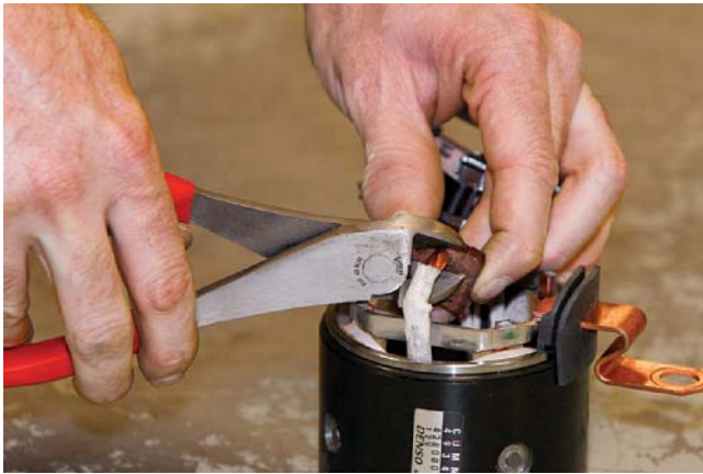
FIGURE 6-29 Removing the worn brushes.
