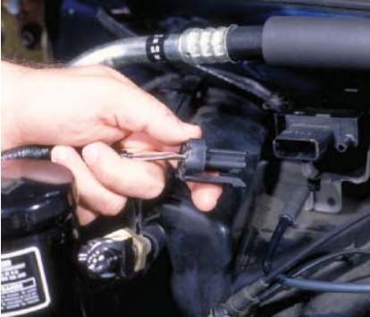
P19-1 Remove the MAP sensor connector and vacuum hose.
