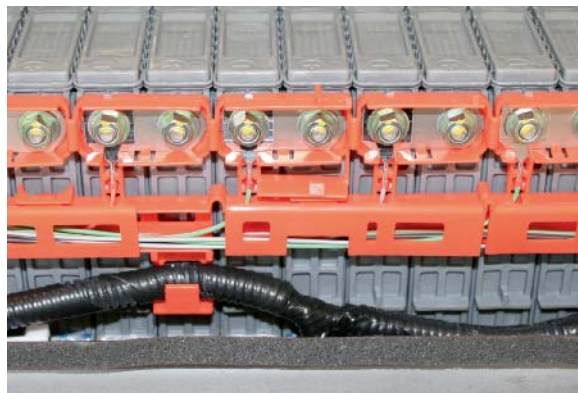
FIGURE 5-22 Cell module connections.
