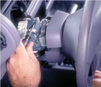
P16-10 Remove the screws attaching the turn signal switch to the lock cylinder assembly.
