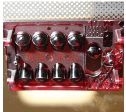
P25-9 Carefully inspect the RSM mounting bracket for any physical damage, including scratches on the RSM bracket lenses. If any damage is found, replace the bracket and windshield as a unit.
