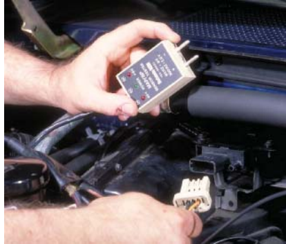
P19-2 Connect the MAP sensor tester leads to the MAP sensor.
