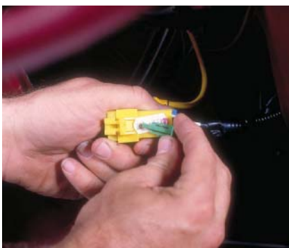
P29-7 Remove the Connector Position Assurance (CPA) from the yellow electrical connector at the base of the steering column.
