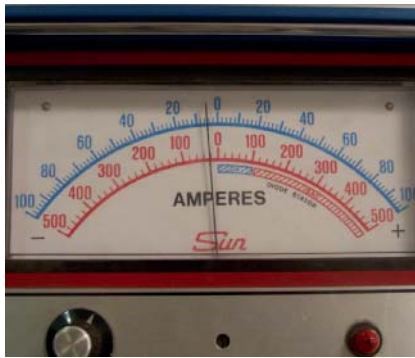
P12-5 With the ignition switch in the RUN position, engine not running, observe the ammeter reading. This reading indicates how much current that is required to operate any full time accessories.
