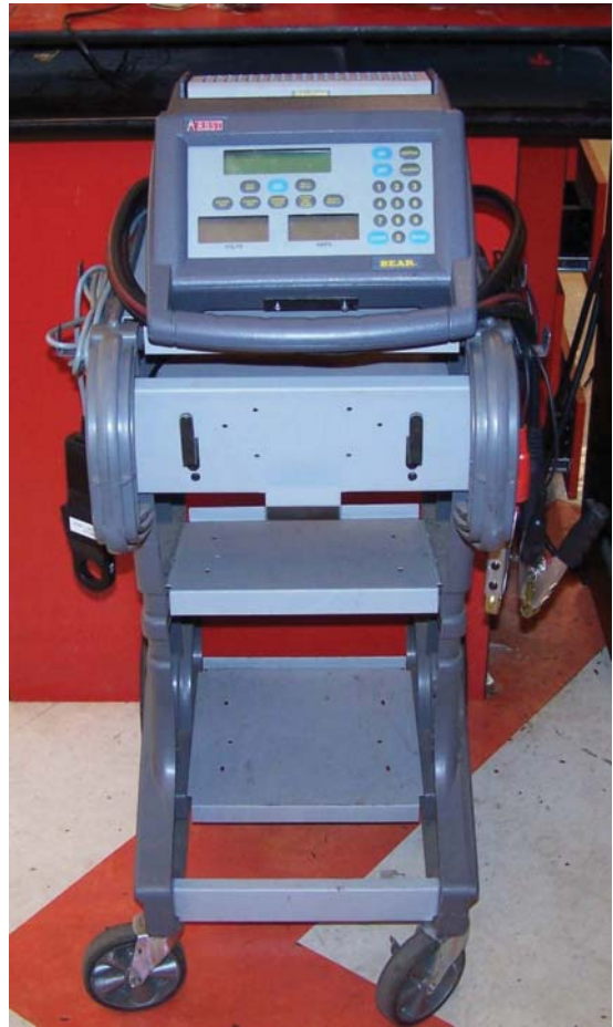
FIGURE 5-2 A computer-based generator, regulator, battery, and starter tester.
