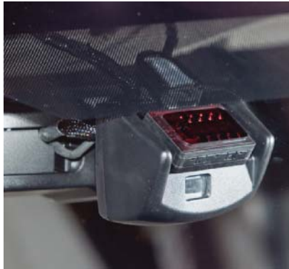
P25-2 From the outside of the windshield glass, carefully inspect the adhesive layer between the windshield glass and the RSM bracket for any voids greater than 0.040 inch (1 millimeter). If an adhesive void is detected, replace the flawed RSM mounting bracket and windshield unit.
