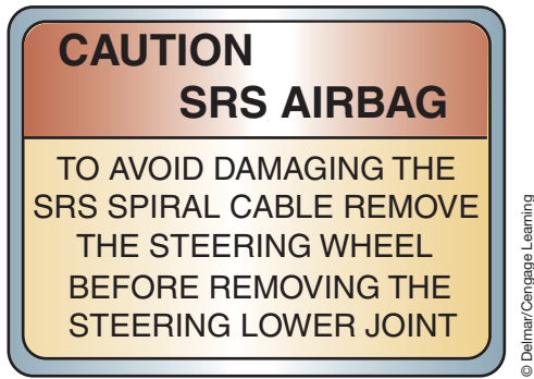
FIGURE 1-26 The air bag wiring and components are usually identified with a warning label.
