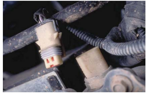
FIGURE 8-42 A combination backup and neutral safety switch installed on an automatic transmission.
