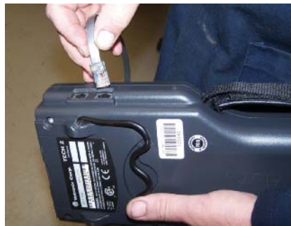
P18-2 Connect the scan tool to a PC that links the scanner to the flash software. Some scan tools will connect directly to an Internet site through a LAN.
