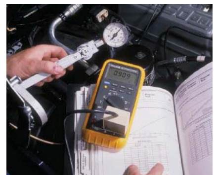
P19-9 Increase the vacuum 20 in. Hg to the MAP sensor and compare the reading to specifications. If any of the MAP sensor readings do not meet specifications, replace the MAP sensor.
