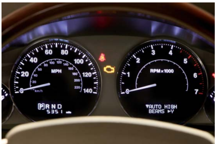
FIGURE 12-14 For the auto headlight system to operate, the drive must activate it.
