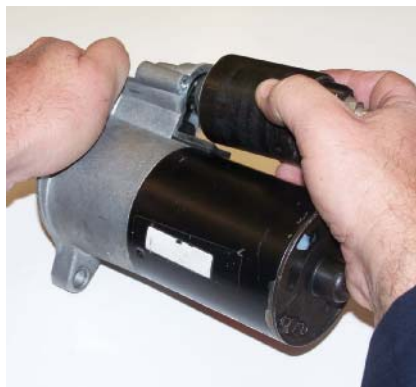
P11-2 Remove the solenoid housing while working the plunger off of the drive lever.
