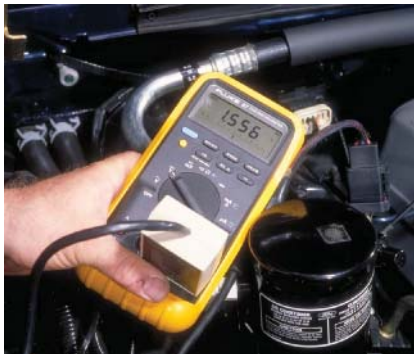
P19-5 With the DVOM set to DC voltage, observe the MAP sensor barometric pressure (BARO) reading on the voltmeter and compare this reading to specifications.
