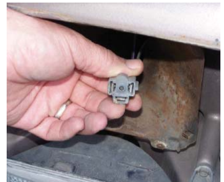
P15-6 Check the wire connector for corrosion or other foreign material. Clean as necessary.
