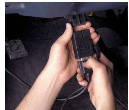
P17-6 Connect the scan tester cable to the DLC and turn the ignition switch to RUN.
