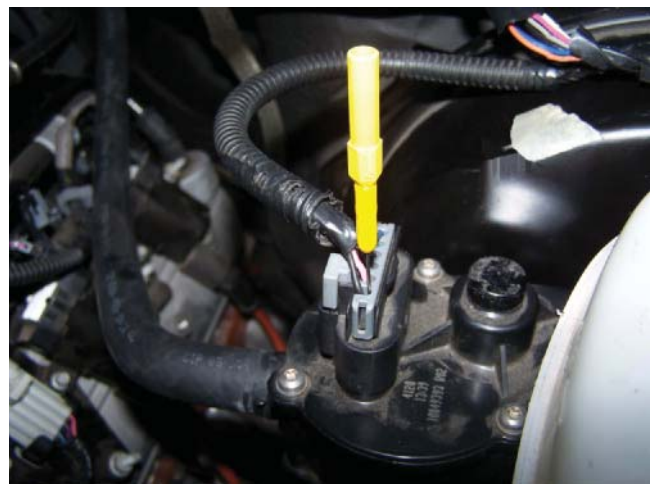
FIGURE 2-15 Backprobing tool properly inserted into the back of a connector.
