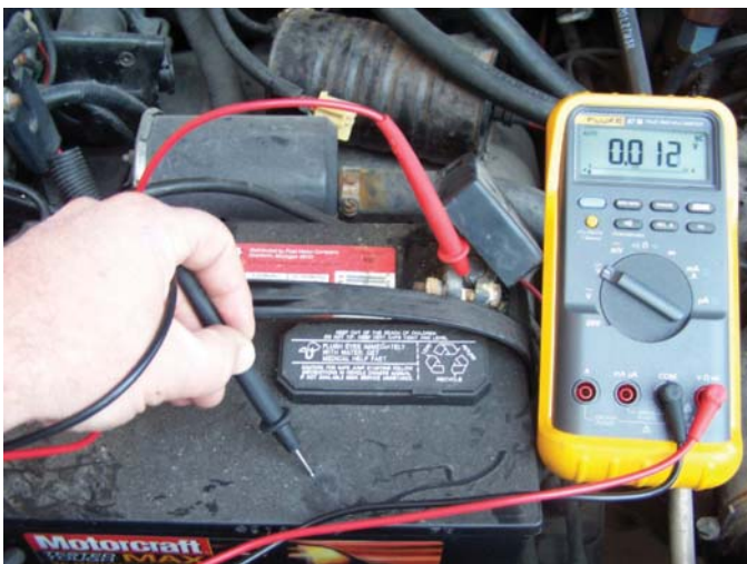
FIGURE 5-10 Using a voltmeter to performing the battery leakage test.
