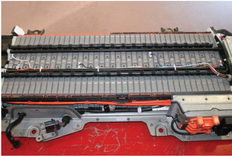
FIGURE 5-30 The modules of the HV battery.
