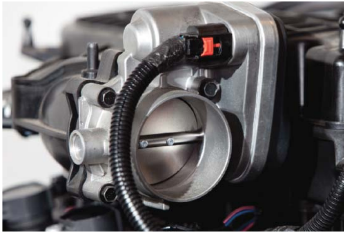
FIGURE 14-79 An electronic throttle control throttle body.
