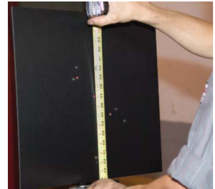
P22-15 Adjust the tripod so that the center LED on the target 57 inches (145 cm) from the floor.
