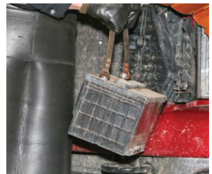
P9-9 Transport the battery to the bench. Keep it away from your clothes.
