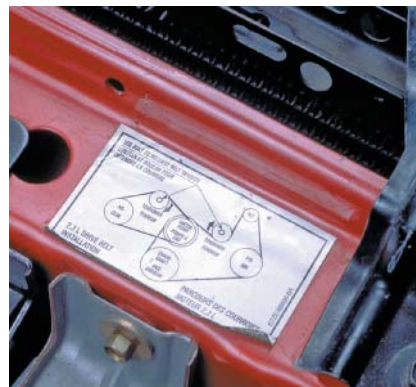
P13-8 Refer to the belt routing diagram that is located on a placard in the engine compartment.
