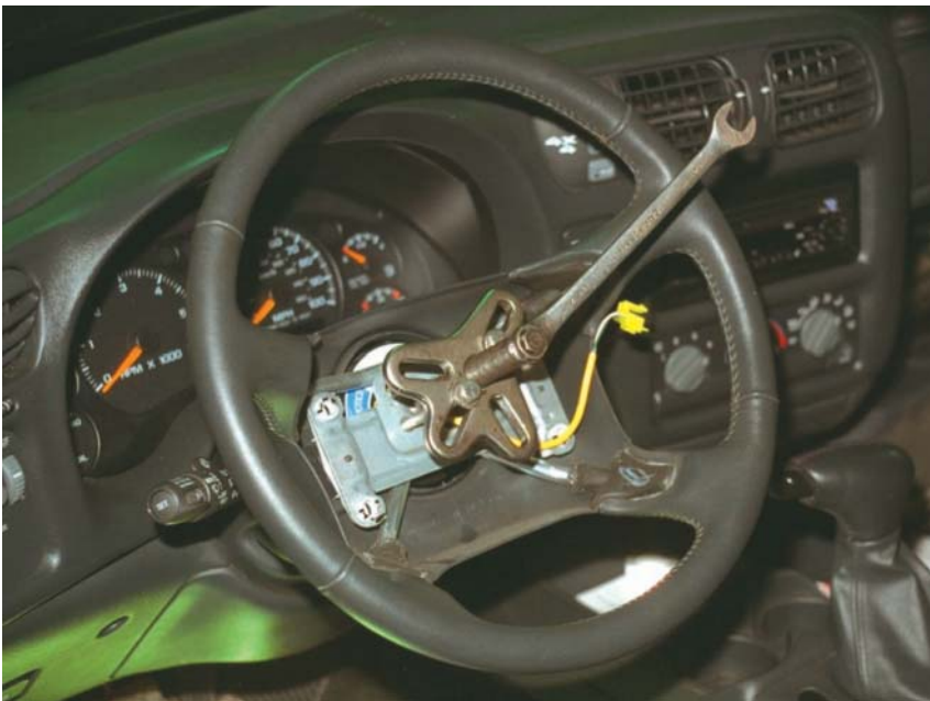
FIGURE 15-7 Removing the steering wheel may require a puller.
