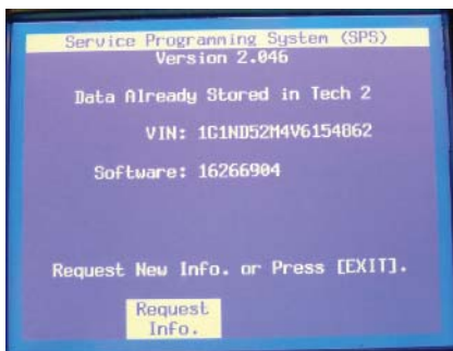
P18-1 Use the scan tool to obtain the part number of the BCM and record the number.
