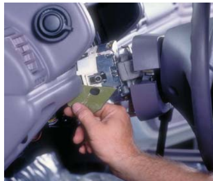
P16-8 Peel back the foam shield from the turn signal switch.
