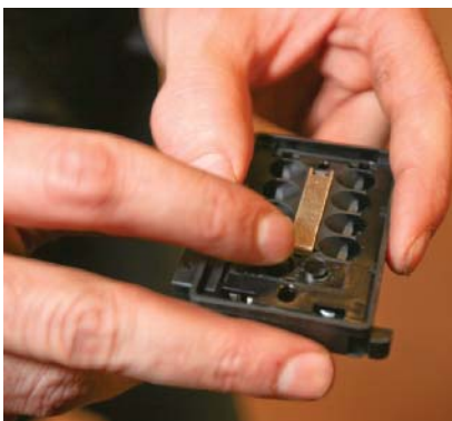
P25-8 Carefully inspect the RSM for any physical damage, including scratches on the RSM lenses.
