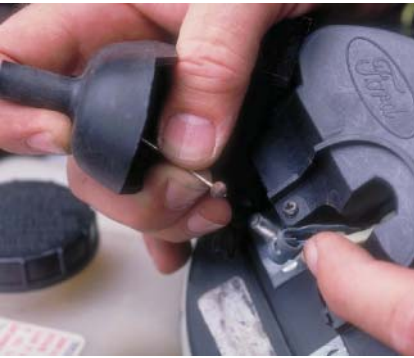
P28-10 Remove the cable from the servo assembly.
