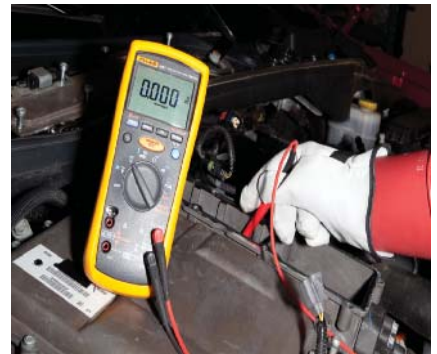
P2-9 Use a DMM to confirm that high-voltage circuits have 0V before performing any service procedure.
