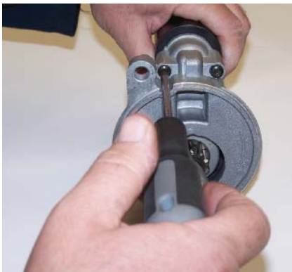
P11-1 Disconnect the lead to the field coil and remove the solenoid retainer screws.
