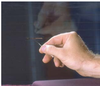
P26-8 Inspect the repair. If it is discolored, apply a coat of tincture of iodine to the repair. Allow to dry for 30 seconds, then wipe off the excess with a cloth.
