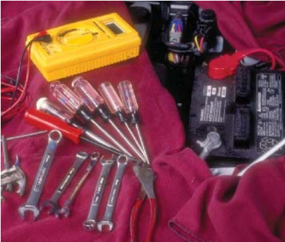
P16-1 Tools required to remove and test the multifunction switch: fender covers, battery terminal pliers, terminal pullers, assorted combination wrenches, torx drivers, and ohmmeter.
