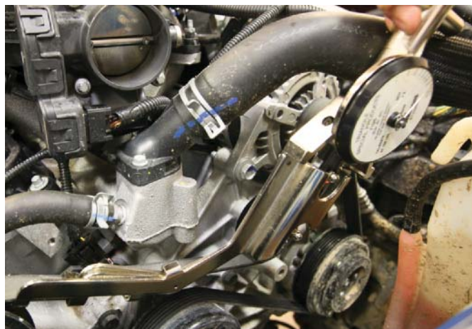
FIGURE 7-2 Checking belt tension using a tension gauge.
