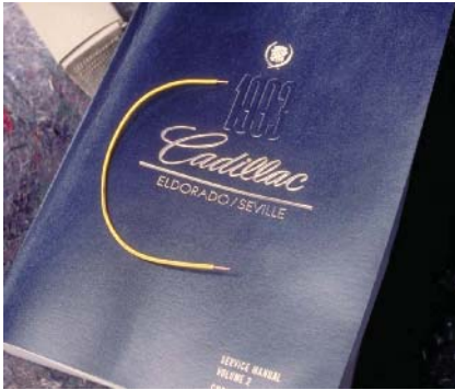
P27-1 The tools required to perform this task are a set of jumper wires and the proper service manual.
