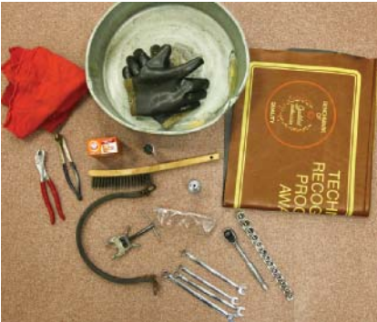
P9-1 Tools needed to remove the battery from the vehicle include rags, baking soda, pan, terminal pliers, cable clamp spreader, terminal puller, assorted wrenches, terminal and clamp cleaning tool, battery lifting strap, safety glasses, heavy rubber gloves, rubber apron, and fender covers.
