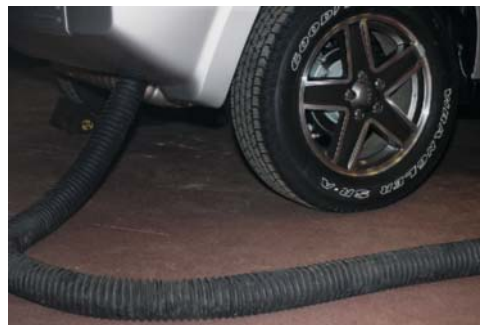
FIGURE 1-17 Connect the ventilation system hose to the vehicle's exhaust before starting the engine. Make sure the hose is secure and there are no kinks in the hose.
