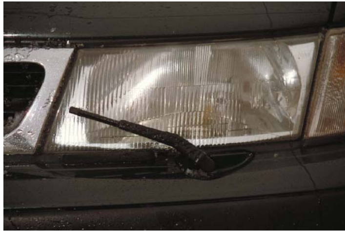
FIGURE 14-27 Headlight washer system may operate with the windshield washer or have a separate switch.
