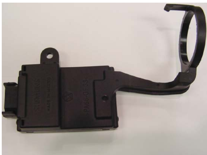
FIGURE 14-72 The immobilizer module with halo antenna.
