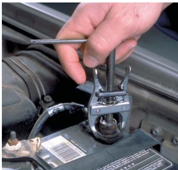
FIGURE 5-8 Use battery clamp pullers to remove the cable end from the terminal. Do not pry the clamp off.
