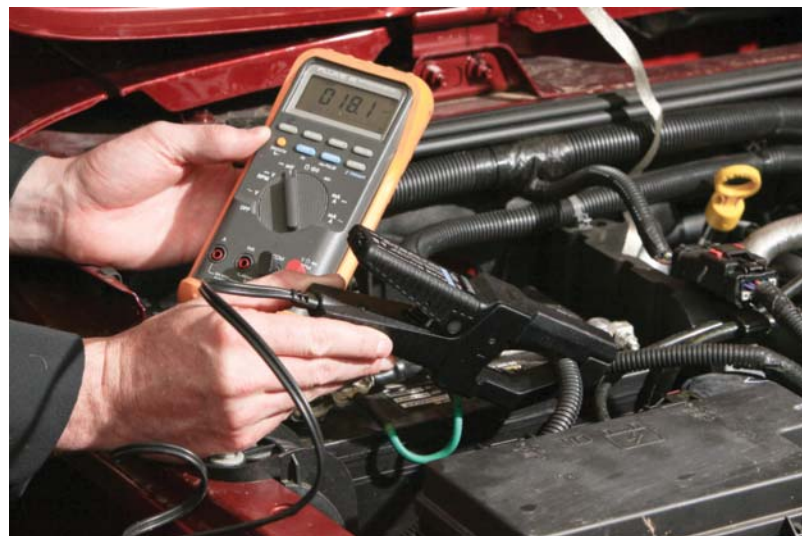
FIGURE 2-19 An ammeter with an inductive pickup. The inductive pickup eliminates the need to connect the meter in series with the circuit.
