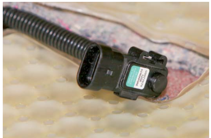
FIGURE 15-39 The pressure sensor changes voltage signals as weight is added to the bladder.
