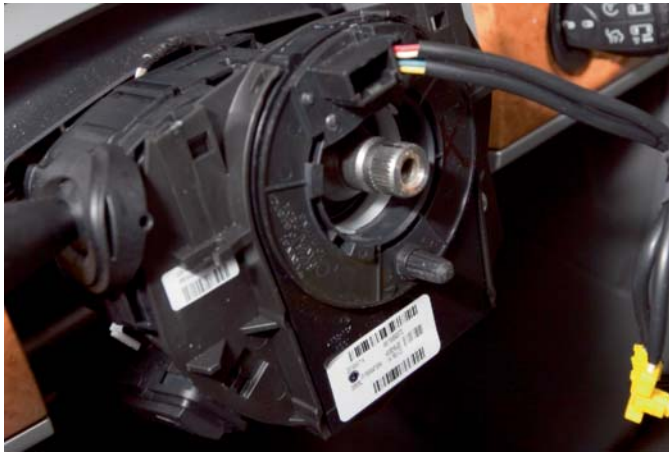
FIGURE 15-12 The clock spring provides for electrical continuity in all steering wheel positions.
