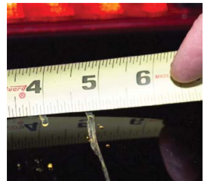
P22-9 Divide the upper measurement in half and mark that dimension on the glass using a grease pencil.
