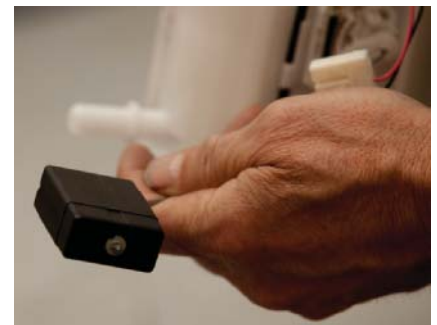
P23-9 Check the float that it is not filled with fuel, distorted, or loose.
