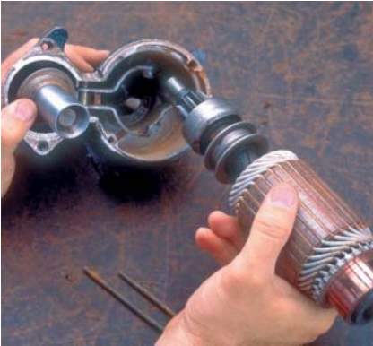
P10-10 Remove the armature from the drive housing. Note: On some units it may be necessary to remove the shift Clever from the drive housing before removing the armature.
