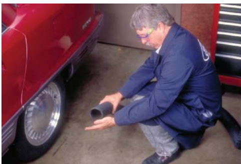
FIGURE 1-16 Testing the ventilation system before using it.
