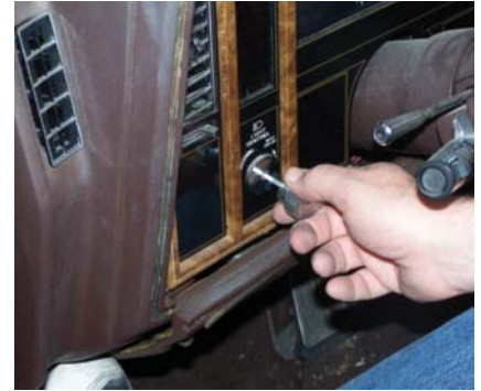
P15-12 Check operation of the headlight.
