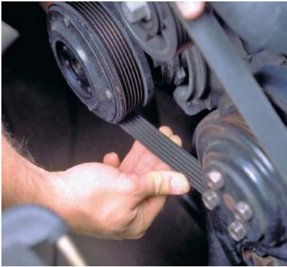
P13-1 Inspect both sides of the belt.
