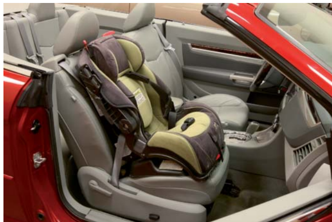
FIGURE 15-29 The BabySmart ® system used by Mercedes automatically deactivates the passenger side air bag when a child safety seat is placed in the front seat.
