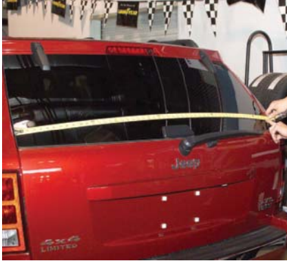
P22-10 Measure across the rear glass at the bottom using the vertical edges of the body opening as the reference points.
