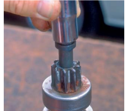
P10-12 Tap end of socket with a plastic hammer to drive the retainer toward the armature. Move it only far enough to access to the snap ring.
