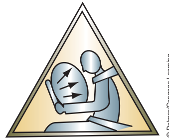
FIGURE 1-27 Some manufacturers identify air bag circuits in their service information with a warning symbol.
