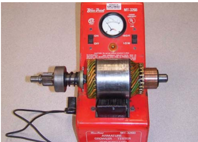
FIGURE 6-22 A growler is used to test the armature for shorts.
