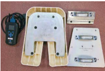
P30-1 Tools required to perform this task include a scan tool and special verification weights.
