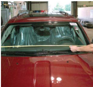
P22-4 Measure across the upper edge of the blackout area at the bottom of the windshield using the inside corner of the intersection between the side blackout area and the lower blackout area as the reference points.
