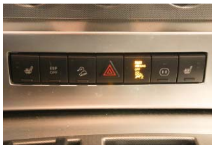
P30-5 Once the test has been started verify that the PADL is illuminated.
