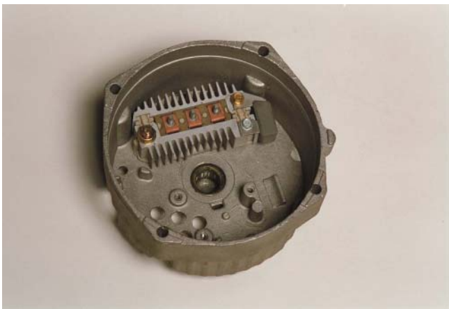
FIGURE 7-20 The positive-biased diodes are mounted into a heat sink to provide protection.
