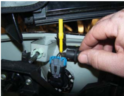
P3-4 Use the backprobing tool to connect the black (negative) voltmeter test lead into the low beam terminal of the headlight socket. Make sure that you are connected to the input side of the headlight.
