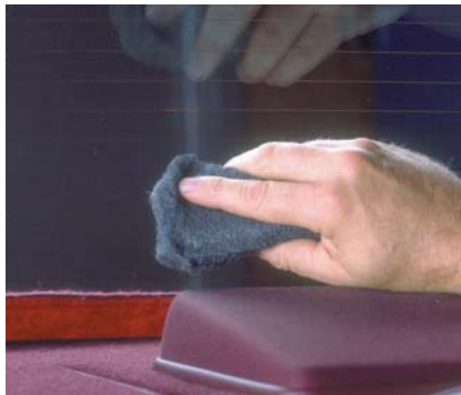
P26-2 Clean the grid line area to be repaired by buffing with steel wool and wiping clean with a cloth dampened with alcohol. Clean an area about 1/4 inch (6 mm) on each side of the break.
