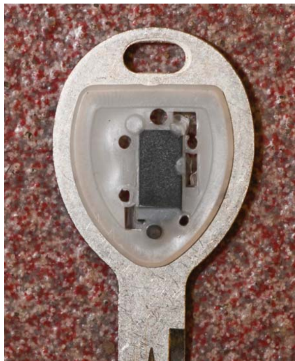
FIGURE 14-73 The immobilizer key has an internal transponder chip. The key cover was cut off for this illustration.
