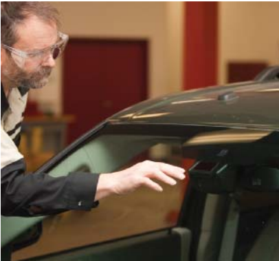
P25-1 Carefully inspect the outer surface of the windshield glass for physical damage, including scratches, cracks, or chips in the vicinity of the RSM mounting bracket lenses. If damage is present, replace the windshield.
