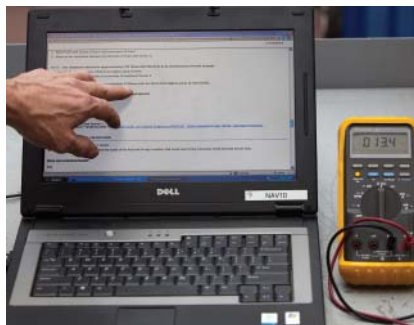
P23-8 Check the resistance value while holding the float against the full stop. Check the results with specifications.
