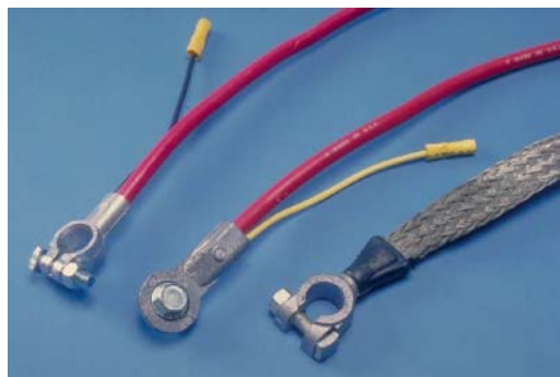
FIGURE 5-27 The battery cable is designed to carry the high current required to start the engine and supply the vehicle's electrical systems.
