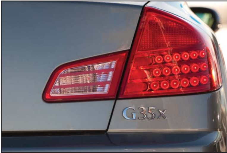
FIGURE 8-37 LED taillight assembly.
