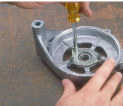
P14-16 Remove the three screws that hold the bearing retainer to the front housing.
