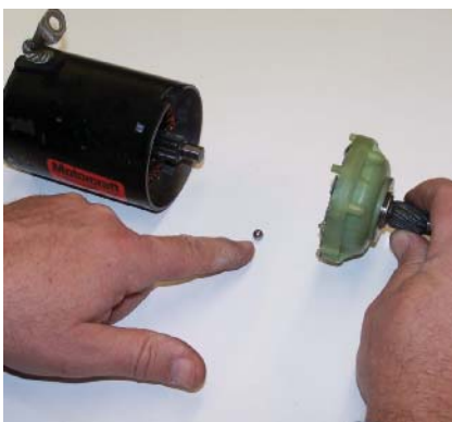
P11-7 Separate the output shaft and stationary gear assembly from the armature. Be sure to locate and retain the thrust ball located in a seat in the output shaft.
