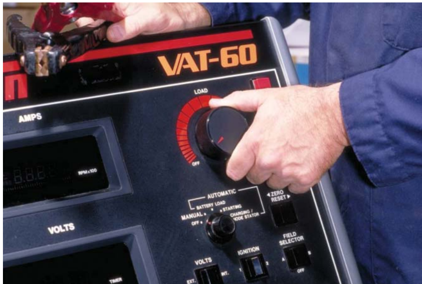
FIGURE 6-4 Starter tests can be performed with any tester capable of measuring high current, such as the VAT-60.
