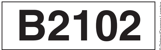
FIGURE 9-8 Example of a body function fault code.
