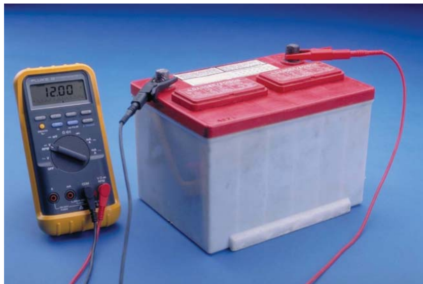
FIGURE 5-17 Open circuit voltage test using a voltmeter.
