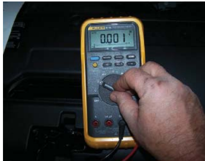
P3-2 Set the voltmeter to its lowest DC voltage scale.
