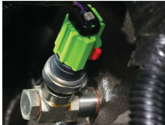
FIGURE 10-11 Oil pressure switch and connector.
