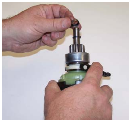
P11-5 Remove the O-ring from the end of the drive gear and then remove the retainer ring and C-clip.
