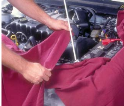
P16-2 Place the fender covers around the battery work area.
