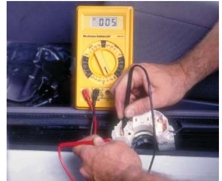
P16-12 Use the ohmmeter to test the switch. Check for continuity from terminal 15 to 13 when the dimmer switch is in the low-beam position.
