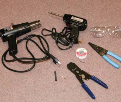
PS7-1 Tools required to perform this task include a crimping tool, splice clip, wire strippers, soldering gun, rosin core solder, heat shrink tube, heat gun, and safety glasses.
