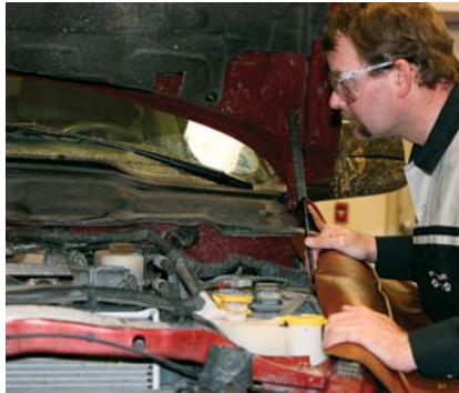
P9-2 Place the fender covers on the vehicle to protect the finish.
