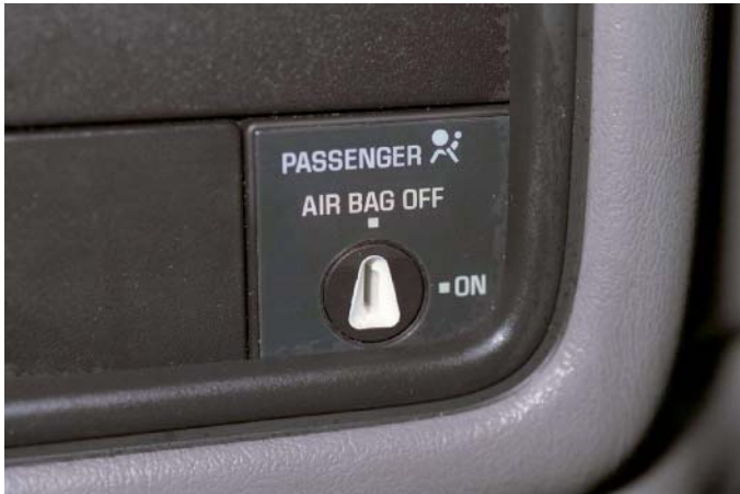
FIGURE 15-30 Passenger side air bag ON/OFF switch.
