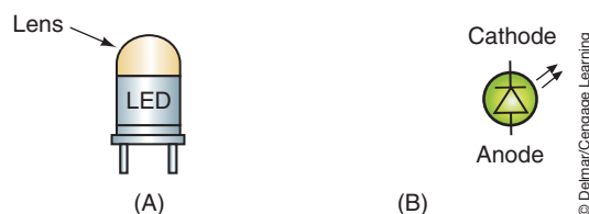
FIGURE 3-25 (A) A light-emitting diode uses a lens to emit the generated light. (B) Symbol for LED.
