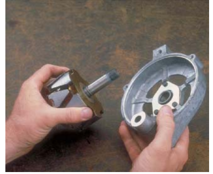
P14-15 Separate the front housing from the rotor. If the stop ring is damaged remove it from the rotor, if not leave it on the rotor shaft.
