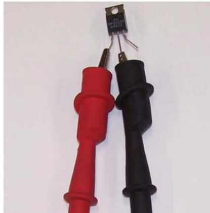
P5-2 Put the positive probe of the DVOM on pin 1 and measure the diode drop to pins 2 and 3.
