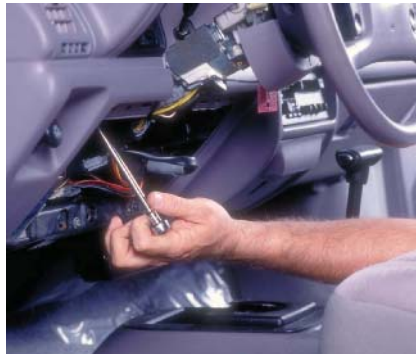
P16-5 If needed to gain access to the upper shroud, loosen the steering column attaching nuts. Do not remove the nuts.
