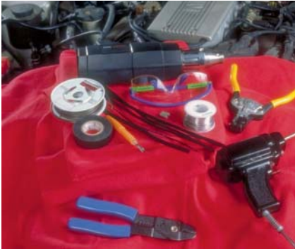
P6-1 Tools required to solder copper wire: 100-watt soldering iron, rosin core solder, crimping tool, splice clip, heat shrink tube, heating gun, safety glasses, sewing seam ripper, electrical tape, and fender covers.
