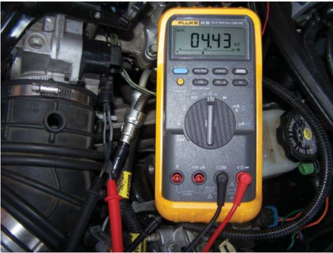
FIGURE 3-29 Using an ohmmeter to test the continuity between terminals A and C of a potentiometer.
