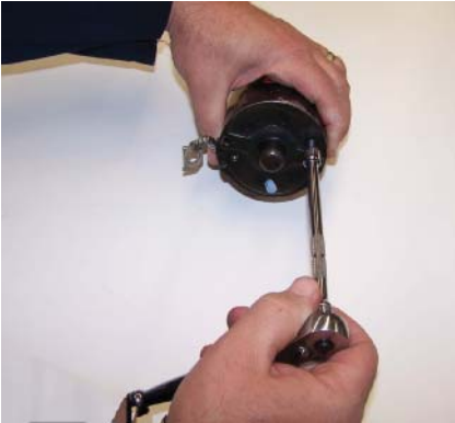
P11-10 Remove the fasteners that attach the end plate to the brush plate.
