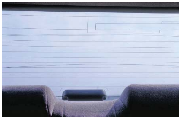
FIGURE 14-37 Rear window defogger grid.
