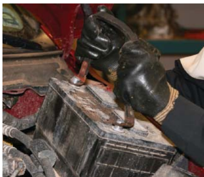
P9-8 Using the battery-lifting clamp, remove the battery out of the tray. Keep the battery away from your body. Wear protective clothing to prevent acid spills onto your hands.
