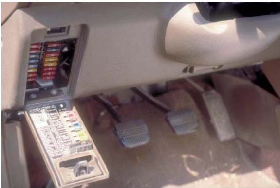
FIGURE 3-44 Fuse boxes are normally located under the dash or in the engine compartment.
