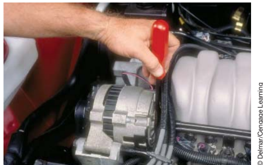
FIGURE 7-10 Quick check of the rotor and brushes.
