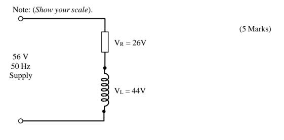
2. Draw to scale the phasor diagram for the following circuit. Include phasors for V<sub>R</sub>, V<sub>C</sub>, and V<sub>S</sub>. <u>*Measure*</u> and state the circuit phase angle.
