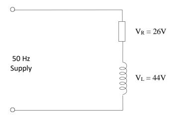
2. Draw to scale the phasor diagram for the following circuit. Include phasors for  $V_R$ ,  $V_C$ , and  $V_S$ . <u>*Measure*</u> and state the circuit phase angle.
