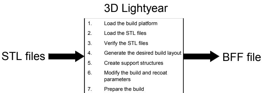
Fig. 1.1 Typical steps used in pre-processing parts in 3D Lightyear
