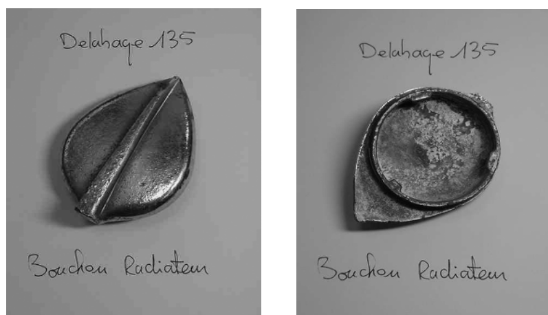
Fig. 9.16 The radiator cap
