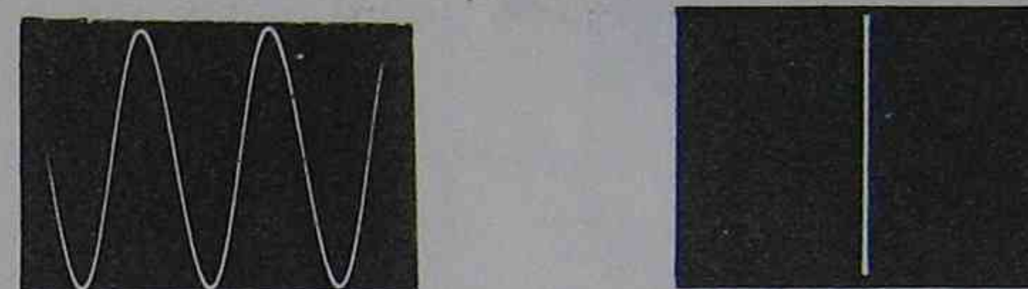
(a) Signal on the Vertical Plates (b) C.R.T. Display with no Horizontal Signal
