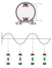
When a two phase a.c. supply is applied to a pair of windings that are displaced by 90°, a rudimentary rotating magnetic field is produced. The field produced by each individual winding pulsates, but due to the 90° displacement, the resultant field rotates. A two phase winding arrangement and the resulting magnetic field are illustrated below:
