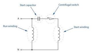
The purpose of the capacitor is to increase the phase shift between the start winding and the run winding. By selecting the correct value of capacitance, a phase shift of up to 90° can be achieved however care must be taken to ensure series resonance is avoided.
