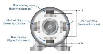
The following diagram shows the physical displacement of windings in a split phase motor.
