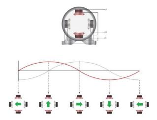
When a three phase a.c. supply is applied to a set of three windings, each displaced by 120°, a smooth rotating magnetic field is produced. Three phase winding arrangements and the resulting magnetic field are illustrated below:
