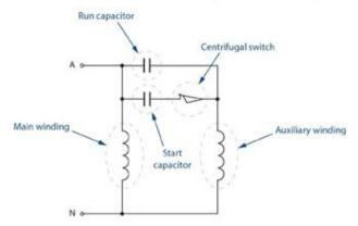
The start capacitor is typically an electrolytic capacitor with a higher capacitance and a short term rating.
