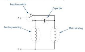
The capacitor must be designed for continuous use, and provides a moderate phase shift resulting in low starting torque and relatively low starting current.
