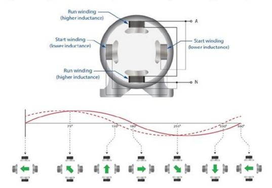
Once the motor is up to speed, the centrifugal switch disconnects the start winding and the rotor rotates purely due to the pulsating magnetic field produced by the run winding.
