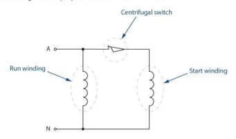
The following diagram shows the electrical arrangement of windings in a split phase motor.
