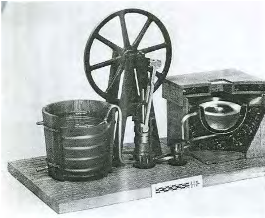
Fig.1.2. Perkins machine built by John Hague
