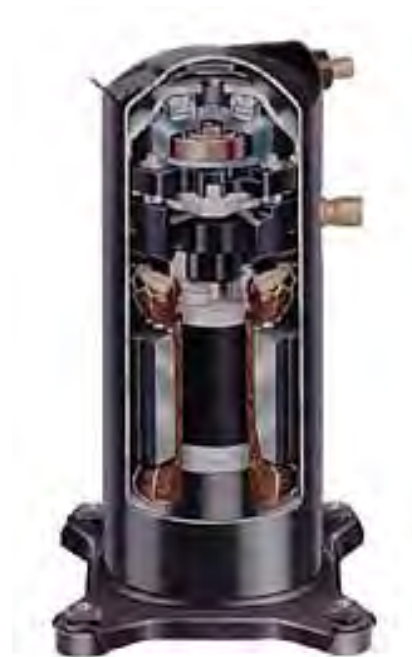
Fig.2.6. Photograph of a cut scroll compressor (Copeland)
