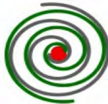
Fig.20.8: Working principle of a scroll compressor
