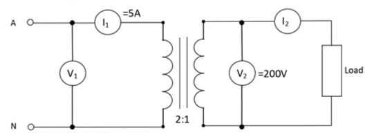
For the single phase transformer circuit drawn above, and using the circuit values shown:
