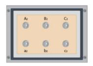
${}^\prime A_2{}^\prime, {}^\prime B_2{}^\prime$  and  ${}^\prime C_2{}^\prime$  are the 'starts' of the three higher voltage phase windings.
