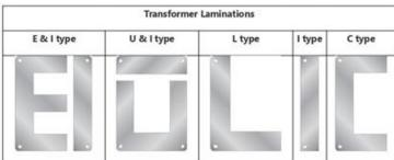
The laminations are stacked in an alternating/overlapping pattern to produce the required shape and thickness.
