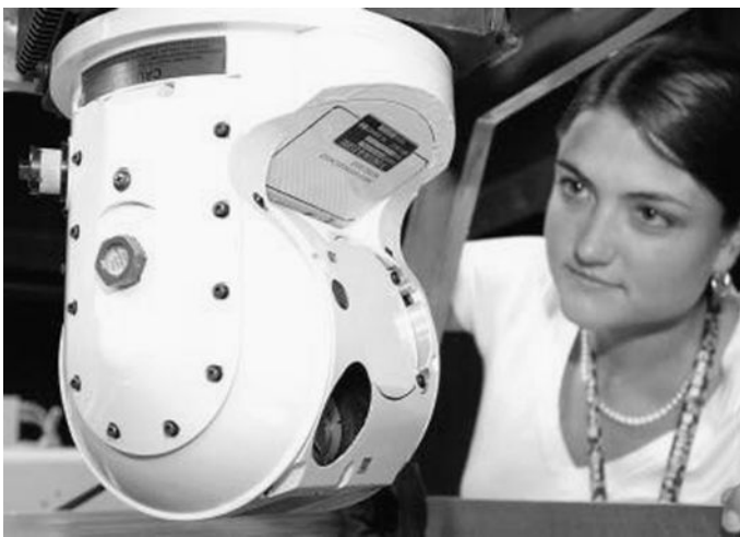
FIGURE 12.11 Turret of built-in BAE Jeteye countermeasure system.
