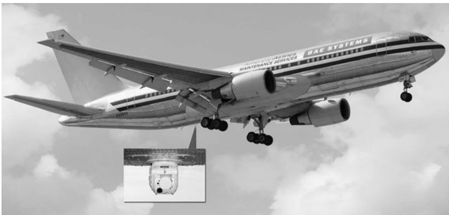
FIGURE 12.12 Testing BAE Jeteye countermeasure system on an American Airlines jet.
