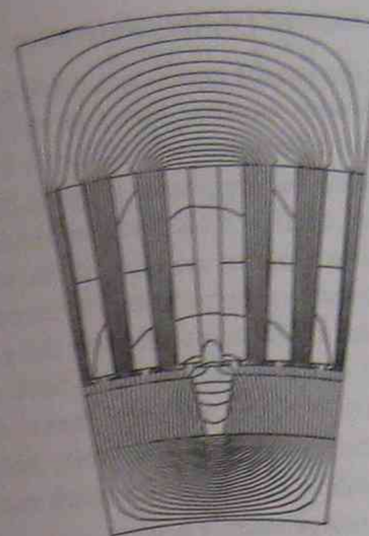
FIGURE 4.9 Flux distribution at no load of a permanent-magnet machine.
