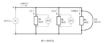
When a short-circuit occurs in a parallel circuit, the total resistance is reduced to almost zero, causing a high fault current to flow. It is the role of a circuit protection device to automatically disconnect the circuit in the event that this occurs. This protects the circuit wiring and equipment from damage due to excessive heat caused by the high current. In this case, total circuit resistance has dropped to less than 0.01  $\Omega$ , resulting in a short-circuit current of over 5 kA.
