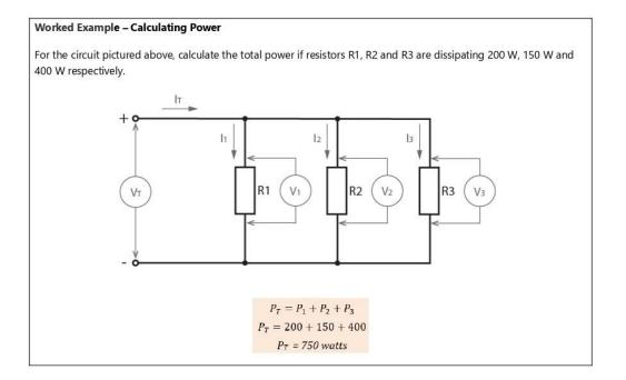
To illustrate how all of these operating characteristics come together, consider the following parallel circuit:
