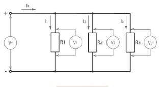
$$R_T = \frac{1}{\frac{1}{R_1} + \frac{1}{R_2} + \frac{1}{R_3}}$$
