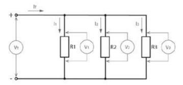
By examining the circuit, it can be seen that *a parallel circuit has several current paths*. When the current reaches a junction, it splits up according to the resistances offered by each path.
