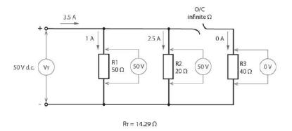
When an open-circuit occurs in a parallel circuit the total current will be reduced. How much the current reduces depends on where the open-circuit occurs. For example, if an open-circuit occurred in the positive wire between the supply terminal and the junction of branch 1, then the total current would drop to zero. In this case, the location of the open-circuit has effectively removed the 40  $\Omega$  resistor from the circuit. The effect of this has been to:
