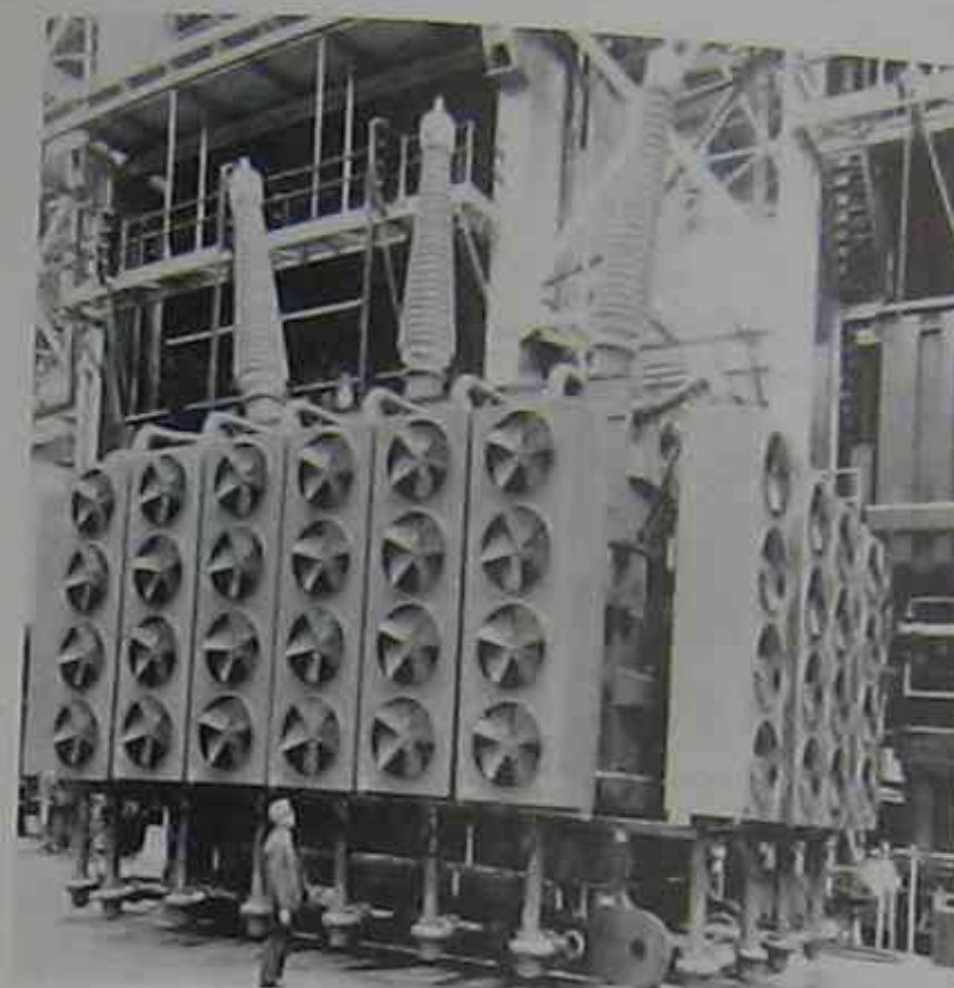
Figure 10.18 Three-phase, type FOA, transformer rated 1300 MVA, 24.5 kV/345 kV, 60 Hz 65°C temperature rise, impedance: 11.5%. This step-up transformer, installed at a nuclear power generating station, is one of the largest units ever built. The forced-oil circulating pumps can be seen just below the cooling fans. (Courtesy of Westinghouse)
