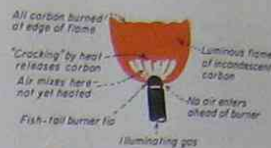
Fishtail gas burner shows yellow flame
