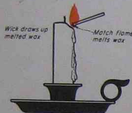
Wick draws up melted wax by capillarity
