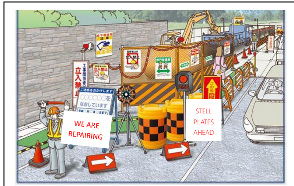
Figure 3.2-3 Occupation of Existing Road with Signboards, Lightings
