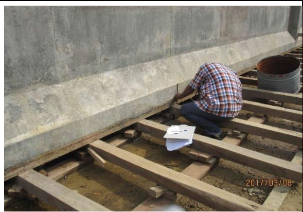
Figure 8.1-8 Measurement of Camber
