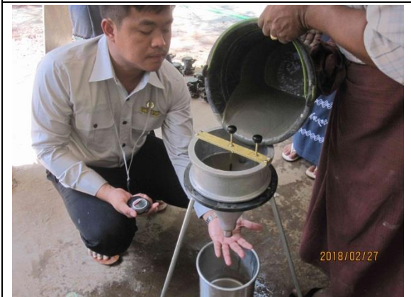
1.1-5 Flow cone testing
