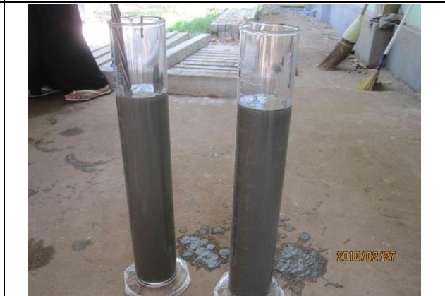
1.1-6 Bleeding and expansion testing
