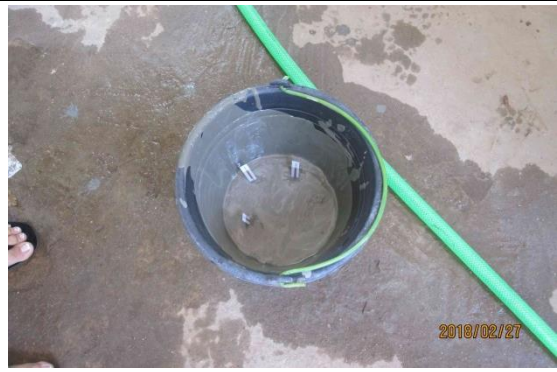
1.1-7 Chloride ion testing
