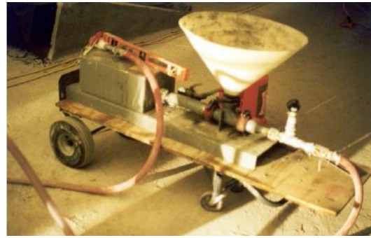
Figure 9.11-3 Vacuum Grout Injection
